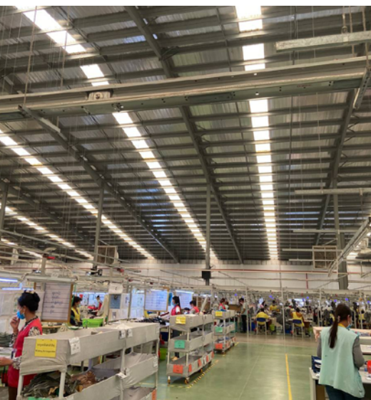
Here, the Cerie factory has adopted a lighting system that uses natural light where possible, improving energy efficiency and workers' well-being
